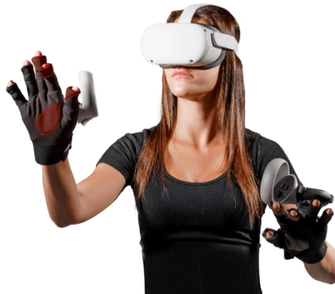
Figure 24. Conductive fabric surfaces used by the smart controller action
