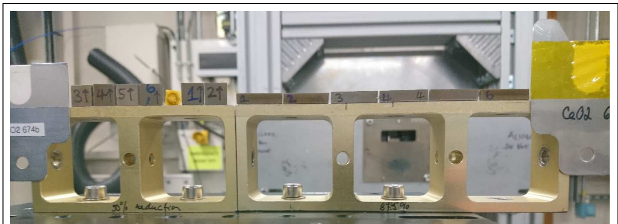
Fig. 2. Ti64 bulky samples mounted on the holder together with CeO2 flat shim samples placed at the edges of the holder.
