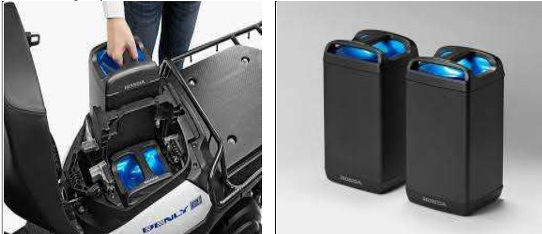
**Fig. 6:-** Swappable Honda E-2W batteries.
