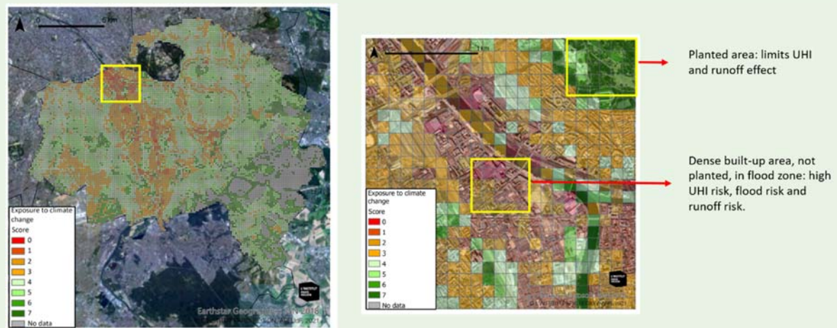
Figure 11: Map of exposure to the effects of climate change in Ivry-sur-Seine and example of interpretation
