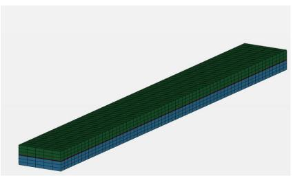
Figure 3. DCB model for Mode I simulation
