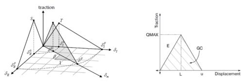
Figure 2. Bilinear Traction-Separation law [10]
