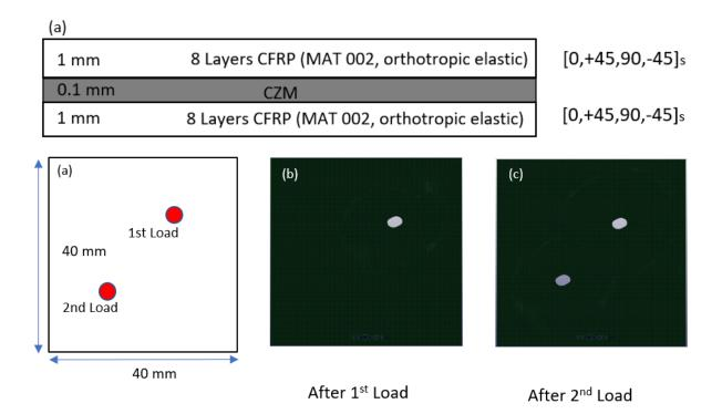
Figure 4. Model geometry (a), Damage pattern from multi-step Laser shock impact. After 1<sup>st</sup> load (b), 2<sup>nd</sup> load (c)
