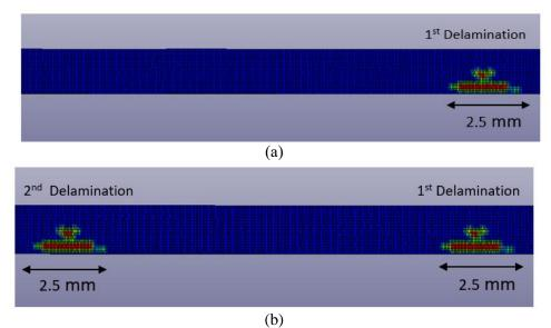
Figure 6. Damage pattern from two-step laser shock loadings, after first load (a), after 2<sup>nd</sup> load (b)
