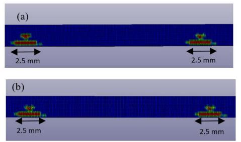
Figure 7. Damage pattern comparison, (a) single model, (b) multi-step model
