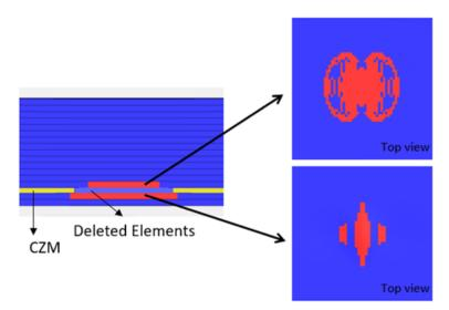
Figure 10. Delaminations caused by laser shock.
