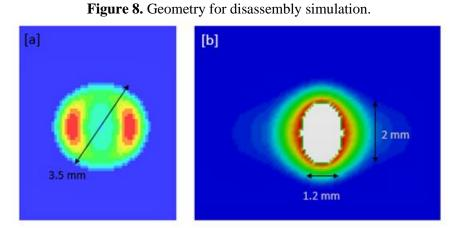
Figure 9. CZM at the loading spot, after the 1<sup>st</sup> load [a], after the 2<sup>nd</sup> load [b].
