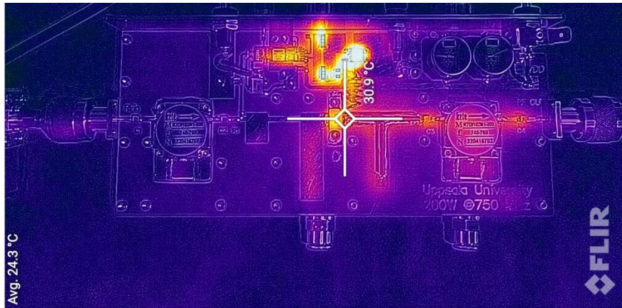
Figure 7: IR camera scan of the 200W power amplifier at 750 MHz.
