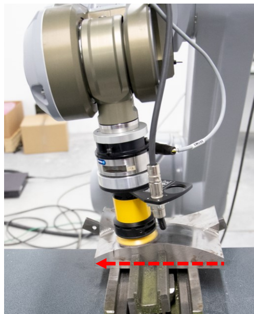
Fig. 9. Spindle orientation capability when programming simple linear paths with vertical spindle orientation (red dotted line).
