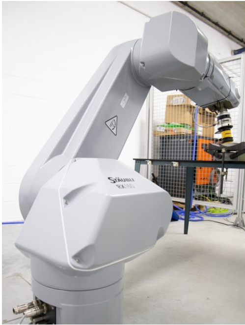
Fig. 7. NC commanded adaptive robotic polishing demonstrator.
