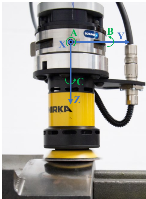
Fig. 8. Integration of the robot wrist, sensor force and polishing spindle, showing force sensor coordinate system.
