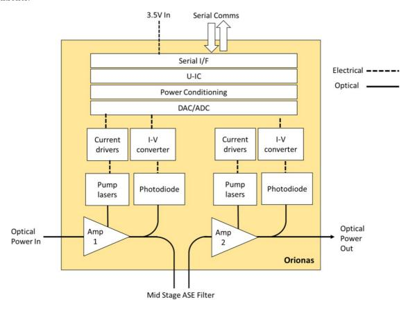
Figure 2. A simplified system level diagram of ORIONAS pre-amplifier design.
