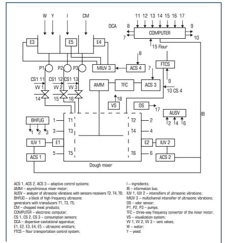
○ Fig. 9.3 Scheme of the experimental unit for preparing dough with ultrasonic intensifiers
