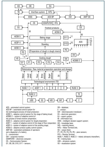
○ Fig. 9.4 Block diagram of a robotic complex for the production of bread
