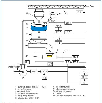
○ Fig. 9.6 Adaptive digital control system for the dough mixing department
