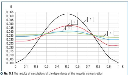
**Q** Fig. 9.2 The results of calculations of the dependence of the impurity concentration in a liquid medium on distance for different moments of time in the numerical solution of the problem:  $1 - \tau = 0$ ;  $2 - \tau = 0.03$ ;  $3 - \tau = 0.06$ ;  $4 - \tau = 0.09$
