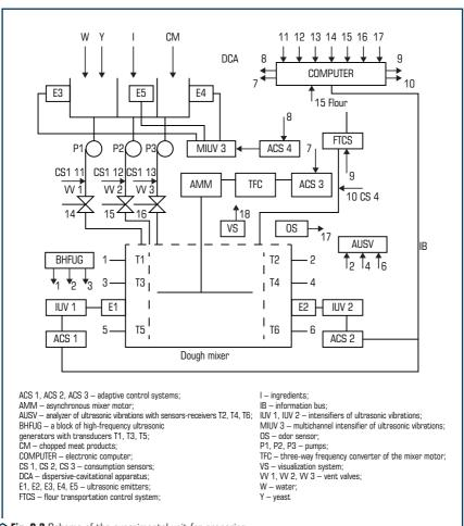
○ Fig. 9.3 Scheme of the experimental unit for preparing dough with ultrasonic intensifiers
