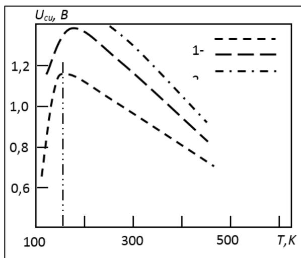
**Figure 2: Calculation results obtained from the expression (12) for the temperature dependence of QE's operating voltage: Calculate the coefficient of non-ideality of VAX 1-n=1; 2-n=1.1; and performed for values 3-n=1,2 [2; pp. 405-410]. Or it can be concluded that the operating voltage will not depend on the non-ideality coefficient of VAX at all.**
