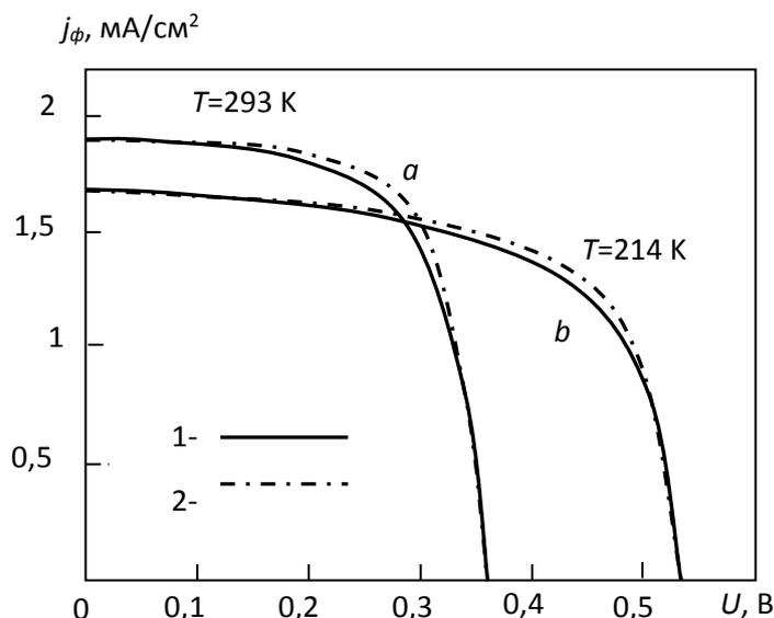
**Figure 4: VAX of hydrogenated amorphous silicon-based QEs at 214K and 293K. Experiment 1 [1; 407 p.] and calculation results obtained from formula (17) when  $\phi_0=0.97$  V,  $j_{00}=3.96 \cdot 10^{-6}$  mA/cm<sup>2</sup>,  $g=5 \cdot 10^{-5}$  eV/K**
