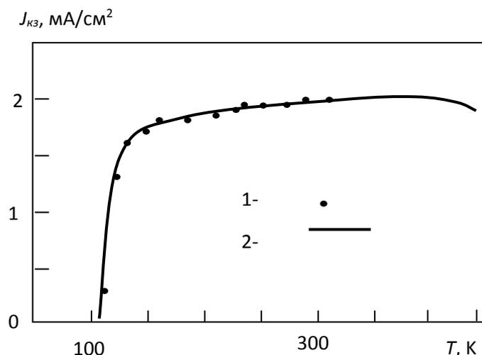
**Figure 3: Temperature dependence of short-circuit current density of hydrogenated amorphous silicon-based QEs. Experiment 1 [1; 217 p.] and calculation results obtained from formula (16) when  $n'=1.006$  and  $\varphi_0=0.97$  V.**
