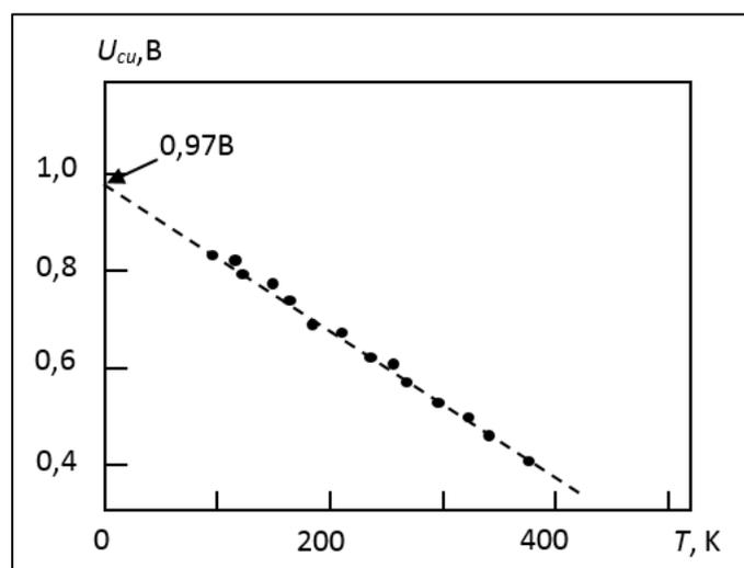
**Figure 1: Experimental results determining the temperature dependence of the operating voltage of hydrogenated amorphous silicon-based QEs ( $U_{i0} = 0.97 \text{ V}$ ) [2; pp. 405-410]**
