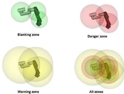
Fig. 3. Blanking, danger and warning zones in joints one, three and five of the ABB GoFa robot. The combination of all zones results in a protective shell around the robot.
