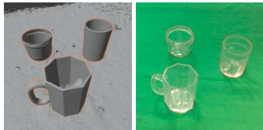
Fig. 5: Outlines of the 3D models (a) are projected onto RGB images (b), allowing the alignment with the object contours.
