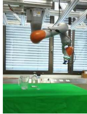
Fig. 3: Setup consisting of a robot manipulator and an RGB-D camera.
