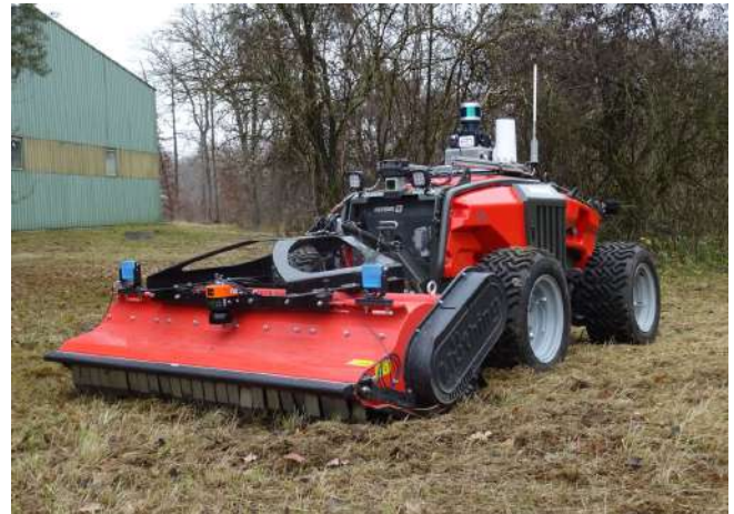
Fig. 1: Carrier platform with attachment and automation kit
