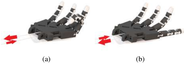
Fig. 2: Flexion (a) and extension (b) of a single finger.
