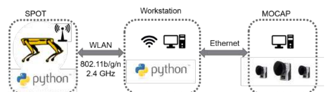
Fig. 2: Software and hardware architecture.
