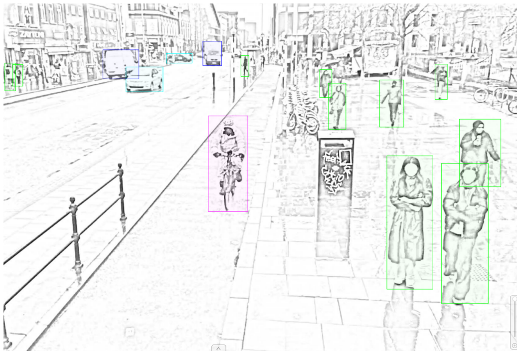
Figure 6: Example of annotated image captured in Manchester. Notice bounding boxes with different colours. Each object class has a unique colour to help minimize mislabelling between classes. Sketch of image to protect privacy.
