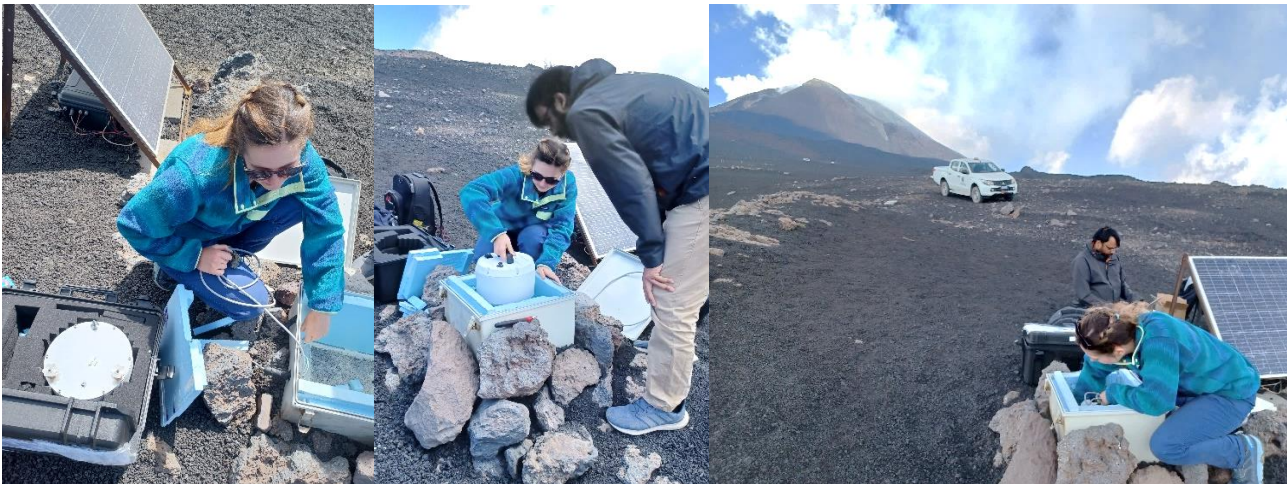
Figure 2 – Deployment of Wee-g7 at EBEL station. The instrument is transported to the installation site upside-down, inside a padded box (left); it is then placed inside the sensor box of the MEMS station (middle; Carbone et al., 2020) and leveled by one operator, while the other checks the effect of turning the adjustable feet of the device through the GUI of the control software (right). The summit craters of Mt. Etna are visible in the background of the picture on the left.
