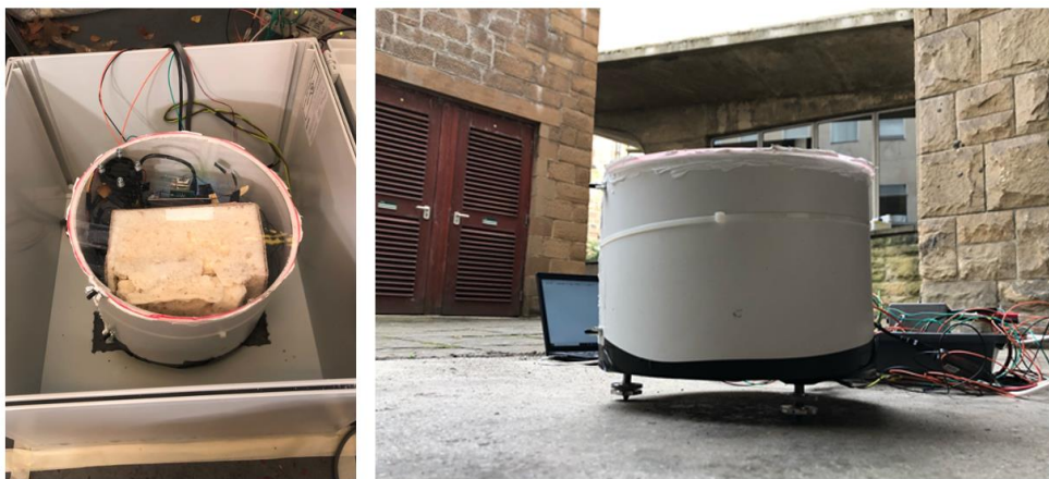
Figure 24 – New test rig setup used for long-term testing of the MEMS gravimeter. The device is housed in a cylindrical enclosure, in order to better replicate the expected final set up.
