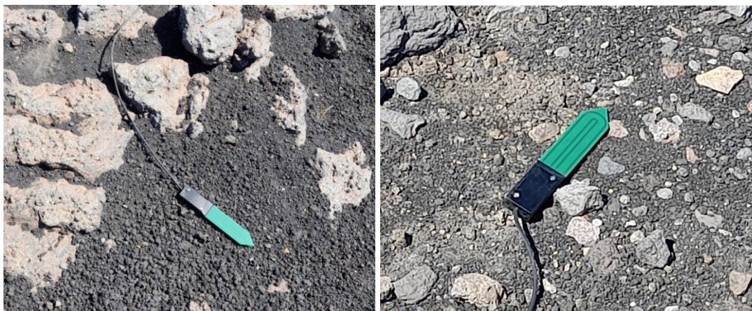
Figure 20 – One of the three soil moisture probes, which is part of the already installed NEWTON-g's MEMS station infrastructure, before it is buried in the volcanic ash at about 20 cm depth.
