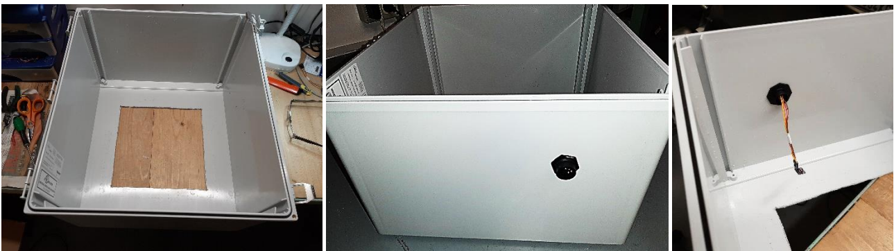
Figure 15 – Phases of preparation of the sensor box prior to installation in the field. A part of the bottom is removed (see text for details) and a panel connector is mounted on one of its sides.
