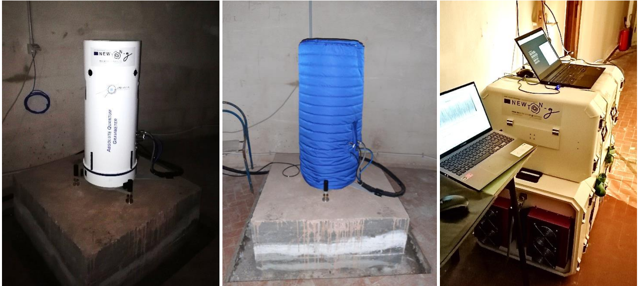
Figure 11 – The sensor head of AQQ-B03 on top of the concrete pillar in the basement of the PDN observatory, without (left) and with (center) the insulation cover. Right: laser and power supply modules in the corridor of the ground floor.
