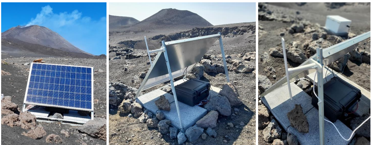
Figure 18 – Left: the foldable galvanized-steel structure, holding the solar panel, installed at the summit of Mt Etna. It is one of the modules that compose the NEWTON-g's MEMS station infrastructure. Middle: four 50 x 50 cm, 20-kg concrete tiles are placed on the base frame of the galvanized-steel structure, in order to enhance its stability against wind. The electronics case is also placed on the base frame of the solar panel structure. Right: detail of the GSM antenna mounted on top of the solar panel structure.
