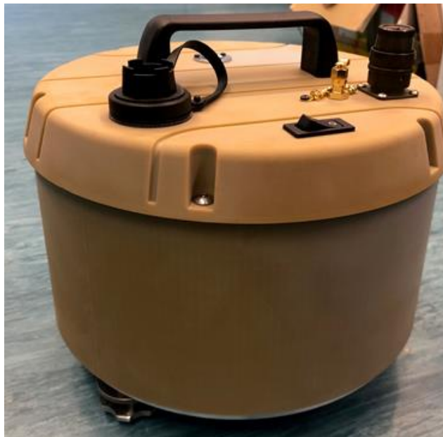
Figure 27 – Prototype field enclosure for the MEMS gravimeter. It is similar to the final version, apart from some characteristics, including the waterproof rating.
