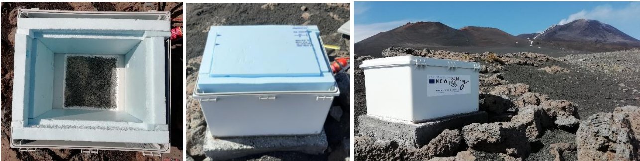
Figure 19 – Sensor box of the NEWTON-g's MEMS station. Left: The bottom of the box is partially removed before installation (see text for details). The sensor box is screwed on the concrete base and sealed with waterproof mastic paste. Middle: 50mm thick polystyrene sheets are used to enhance thermal insulation. Right: the sensor box after installation.
