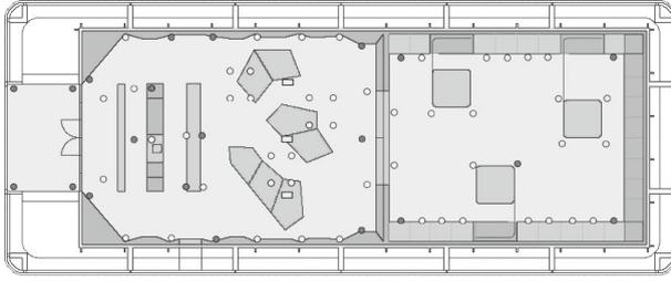
**Fig. 5.** Positions of the 70+ ultrasound receivers in the iHomeLab. The inner gray rectangle indicates the covered area (about  $10m \times 30m$ ). The iHomeLab is located at Lucerne University of Applied Sciences at Campus Horw.
