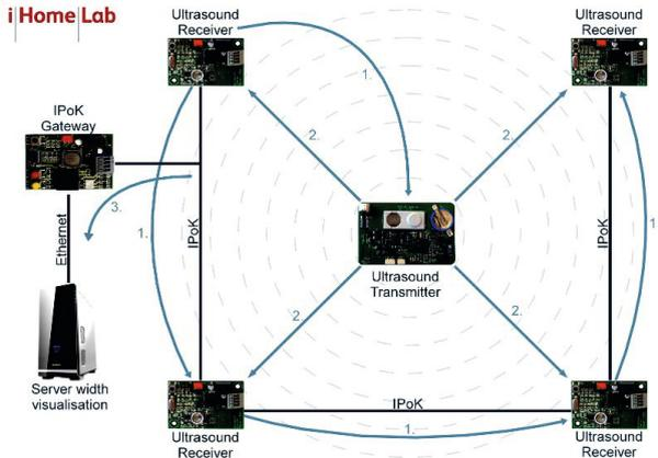
**Fig. 1.** Setup overview: Four reference nodes are shown. The upper left receiver sends out a synchronization signal (arrows labeled “1”) by wire (“IPoK”) to the other reference nodes and by radio to the mobile node (center). The mobile node emits an ultrasound pulse (arrows “2”) and the reference nodes record the reception time.
