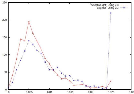
**Fig. 10.** Observed position error in a lab environmet after careful adjustment (not the EvAAL setup): dashed line (blue, \*) indicates positions which were obtained by multilateration. Solid line (red, +) indicates positions calculated with trilateration and a selection algorithm. X-Axis: error [meters], Y-Axis: number of samples [7].
