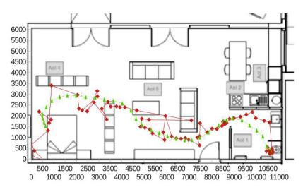
Fig. 8. Positions obtained for a specific test during the competition at CIAMI Living Lab. Bright/yellow triangles indicate real path, dark/red diamonds indicate iLoc results.
