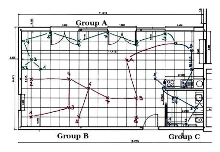
Fig. 7. Positions of the 28 iLoc receivers at CIAMI Living Lab. The nodes are arranged in 3 wiring groups, as indicated in the image.
