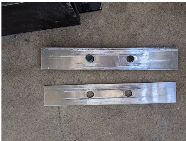
Fig. 12. Aluminium shim layers after the tests.
