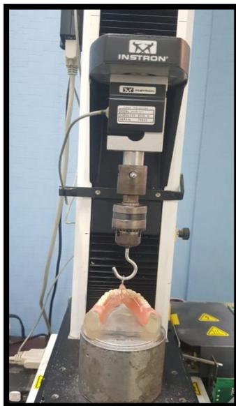
**Figure 9: The Instron universal testing machine**
