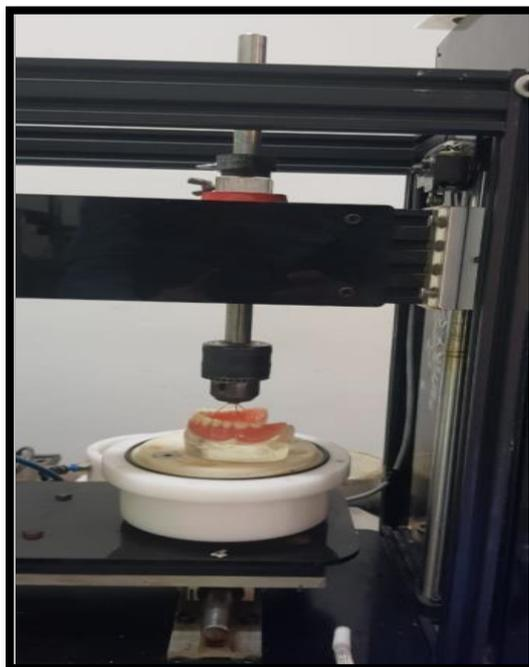
**Figure 10: ROBOTA chewing simulator**
