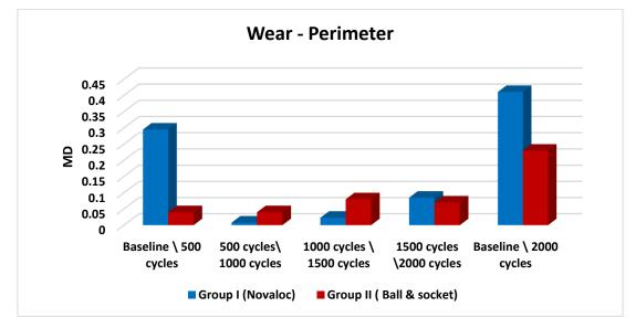
Figure 12: Mean difference of wear – perimeter of both groups
