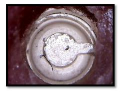
Figure 19: after 2000 cycles Group II Ball attachment:
