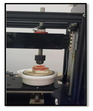
Figure 10: ROBOTA chewing simulator
