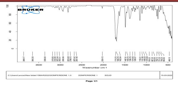
FTIR spectra for pure domperidone and in combination with the polymers(DBF6) Discussion: the spectra for pure drug and optimized formulation showed that there is no interaction of drug with polymers.
