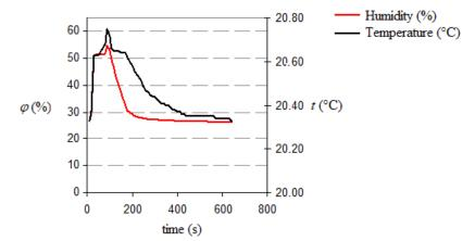
FIGURE 9: Dependence of relative humidity and temperature of unground silica gel at measuring point B
