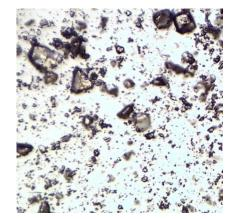
FIGURE 4: The structure of silica gel under a microscope
