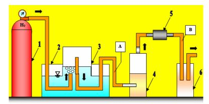
1 – pressure vessel, 2 – outer container, 3 – measuring cylinder, 4 – container with silica gel, 5 – filter, 6 – drain container SiO<sub>2</sub> FIGURE 5: Model of experimental equipment
