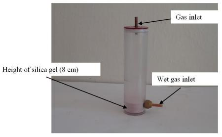
FIGURE 6: Vessel with silica gel
