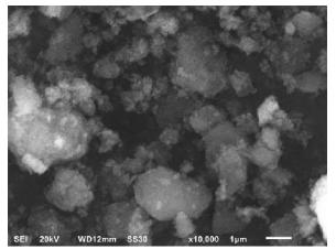
FIGURE 1: Structure of silica gel [6]
