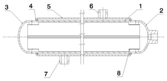
cylindrical part of the primary vessel, 2- elliptical bottom with NPT1/4"thread,
