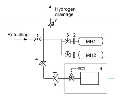
MH1 and MH2 represent the used MH vessels within the design, 1- refuelling neck, 2- filter, 3- manual valve, 4 - Solenoid valve, 5- reducing valve, 6- fuel cell and regulation, 7- hydrogen drainage. FIGURE 4: Hydrogen circuit in designed two-wheeler
