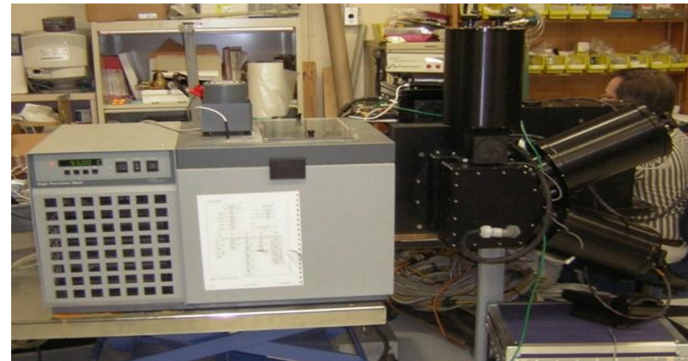
M-AERI is calibrated in the laboratory before and after each deployment using an external validation procedure.
