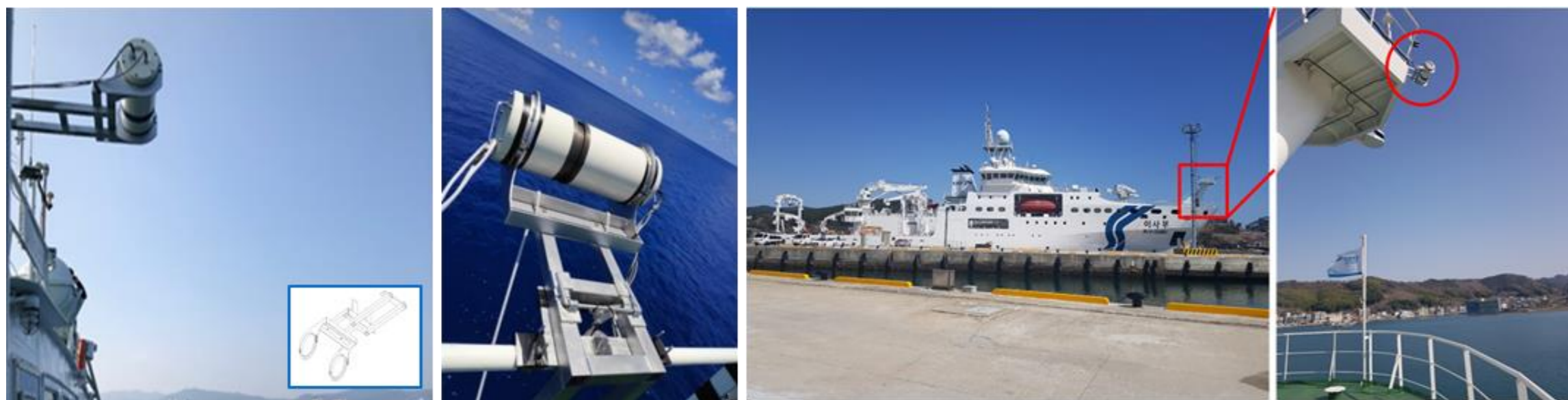
▲ Figure. Schematics of designs of the shipboard mounting system for a folding style and a sliding style fitted to the conditions of each vessel, and the features of ISAR mounted on guardrail of the ship for measurement tests on R/V ISABU.
