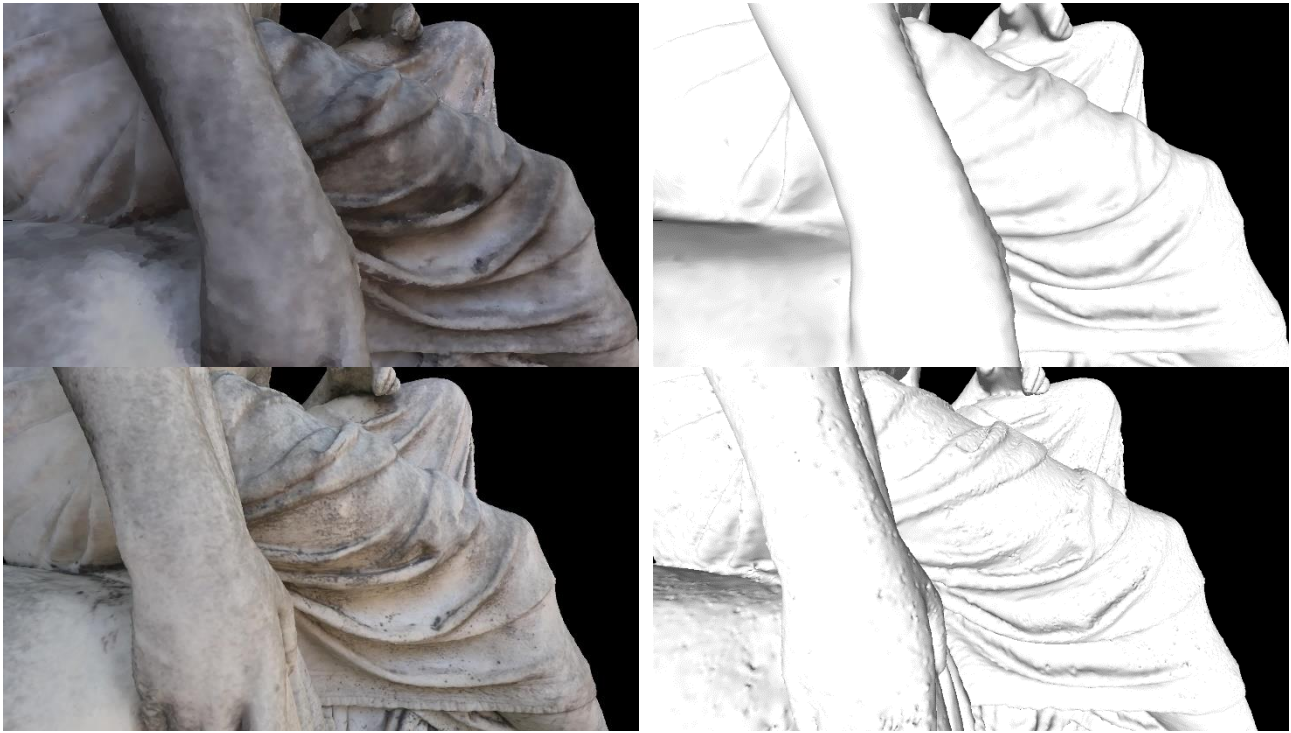
Figure 9. Comparison of handheld scan (top) and photogrammetry (bottom).
