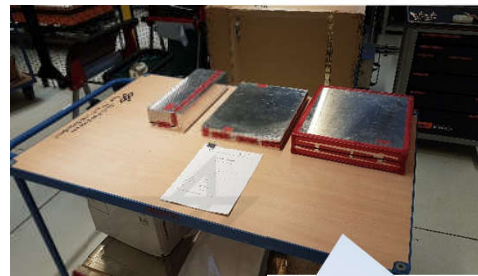
Cured in Autoclave
