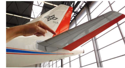
Horizontal Tail-Plane (HTP) Leading Edge on a A320
