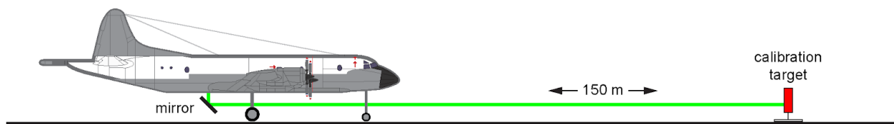
Figure 3: Range bias determination (a.k.a. ground test) using a calibration target with a known distance. The distance to the calibration target is measured with an electronic distance meter (a.k.a. “total station”) with an accuracy of a few mm.
