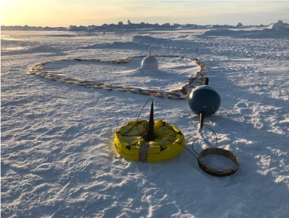
Figure 7: The white ice buoy (APL-UTAP-0039) surrounded by the wooden boats from “Float Your Boat”. In front the SVP-B buoy (60712070). These buoys can be followed at the following link: https://iabp.apl.uw.edu/IABP_Maps.html
