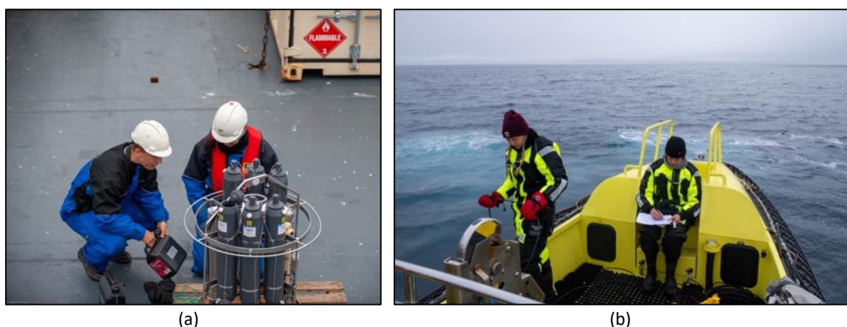
Figure 4: Students recovering water samples taken with the rosette on the CTD (a), and doing acoustic transmissions from the small boat (b).
