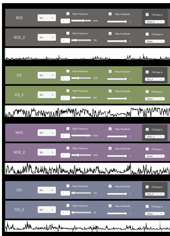
Figure 4. The configuration to replicate the sound design of the sonification of air quality data, where the first row of each data attribute serves as the modulator, and the second is the carrier for FM synthesis.
