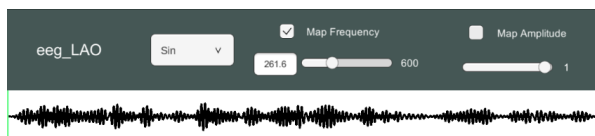
Figure 2. Frequency modulation by EEG data with a minimum frequency of 261.6 Hz and a frequency range of 600 Hz.
