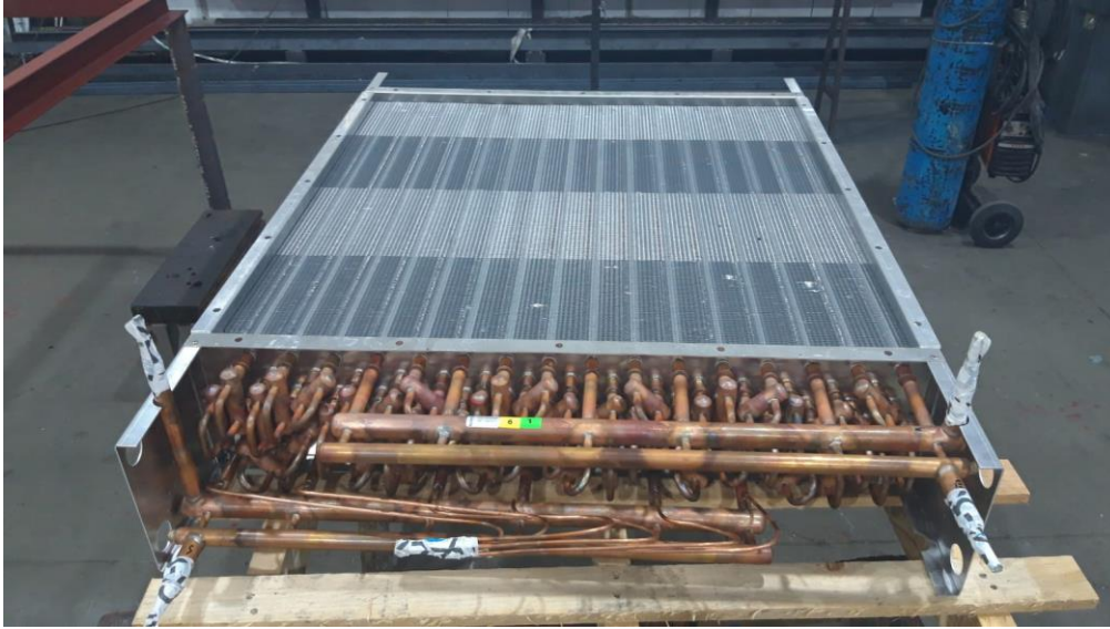
Figure 1. Dual source Heat exchanger (DSHX) prototype
