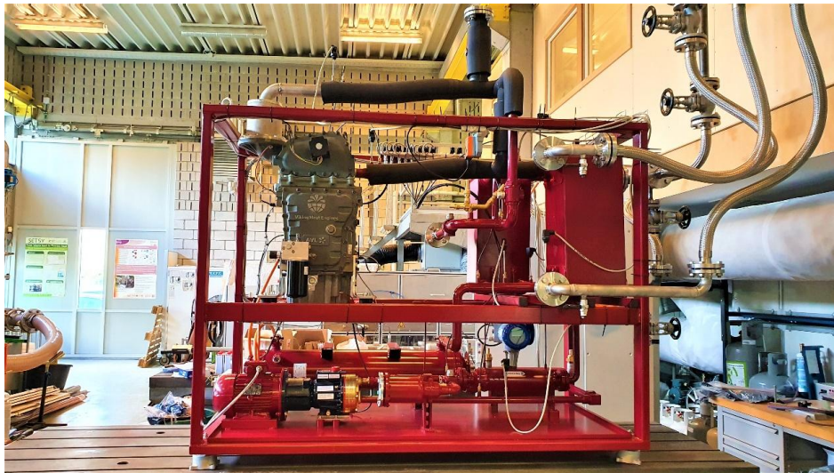
Figure 5: ORC prototype experimental test rig
