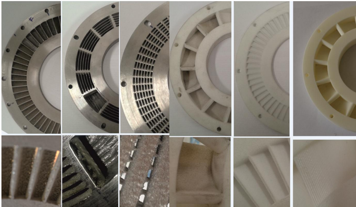
Figure 3: Investigated 1 st gen stator wheels, from the left – DMLS as-printed short chord stator, DMLS polished long chord stator and DMLS stator with the functional supports, SLS long chord, SLS short chord, FDM long chord
