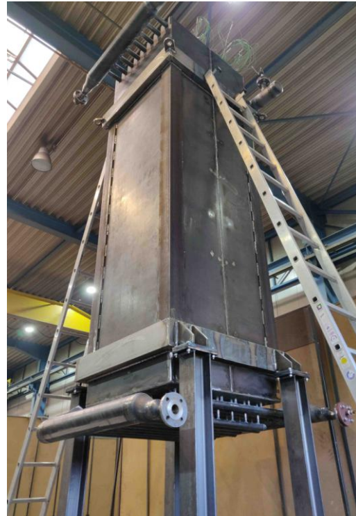
Figure 11: Technical drawing of the final storage design (left) and LH-TES during manufacturing (right)
