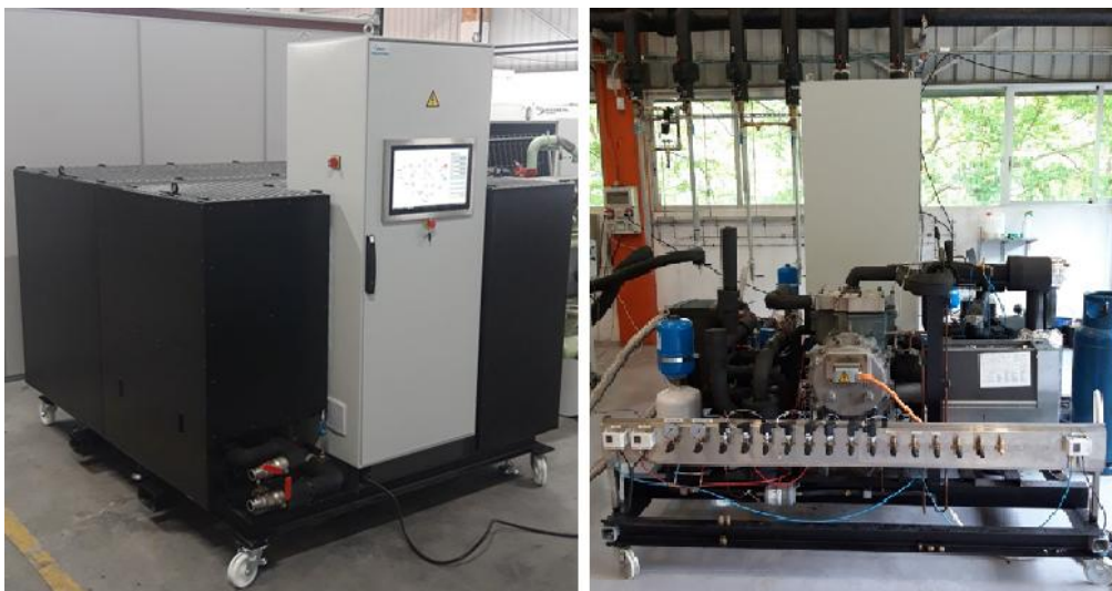
Figure 2: Overview of the HTHP unit with/without the protective casing
