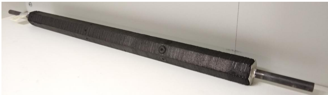
Figure 1: Carbon-aluminium fin laminate over a 10 mm O.D. stainless steel tube
