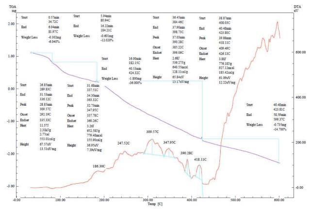
Thermal analysis of the complex compound [Cu(L)2]. The complex was studied at temperatures up to 600°C.
