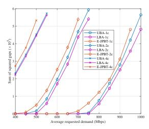
Fig. 6: The gap performance value with respect to traffic demand of the proposed BH-NOMA schemes in different scenarios with 1-color, 2-color, adn 4-color frequency-reuse patterns.
