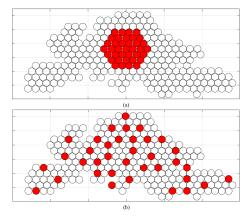
Fig. 2: Beam pattern covering Europe provided by ESA [23] and the adopted two scenarios, where BH is operated among the considered 37 beams (highlighted in red color).
