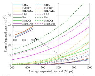
Fig. 5: The gap performance with respect to traffic demand among the proposed schemes and benchmarks. (Scenario 1, 5 terminals per beam,  $K_0=3$ ) (Solid line: under free-space channel model [3], [6], [10]; Dash line: atmospheric channel model with long-term effects and rain effects [40].)
