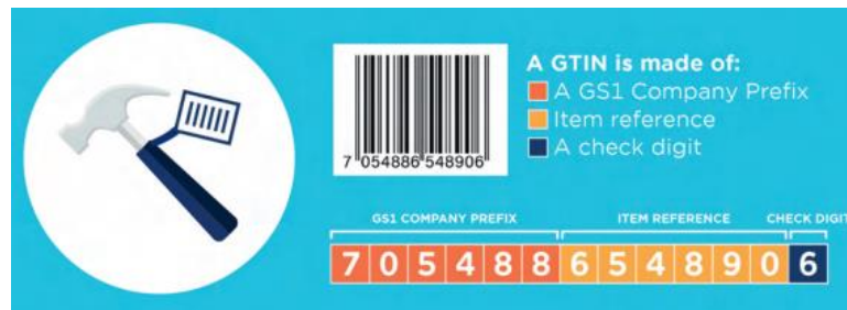
Figure 8: Example of the structure of GTIN-13 with 6-digit GS1 Company Prefix
