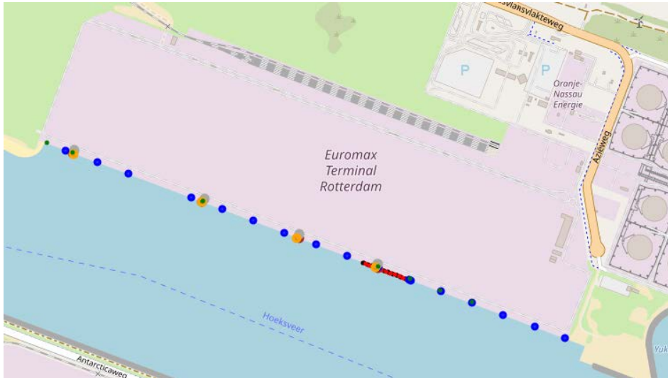
Figure 11 Positions of fibre optic sensors of PUC10 Quay wall
