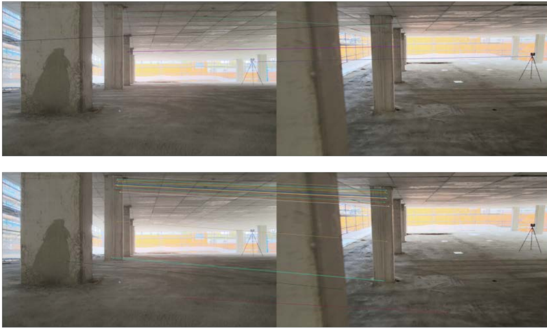
Figure 18: Example of SIFT and D2-Net feature matching in two images with poor overlap from Demo Site #6 indoor dataset a) at the top is presented the SIFT matching with 314 raw matches and 9 inliers detected for the matching, b) at the bottom image the D2-Net performs better with 1627 raw matches and 23 inliers for the matching.
