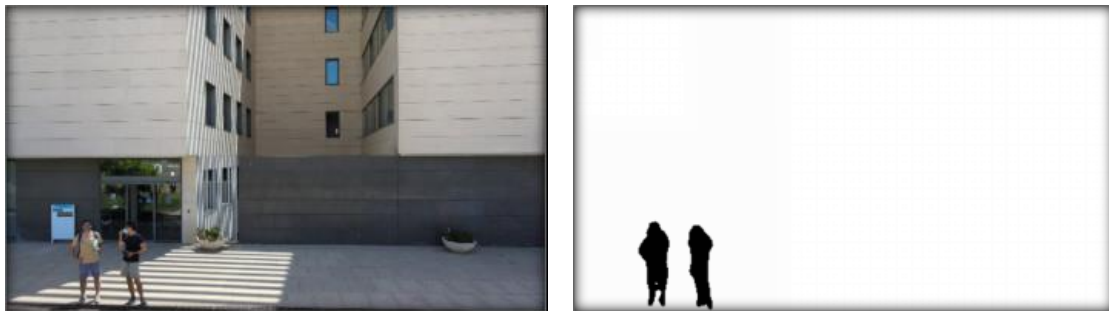
Figure 4: Masking results of the DeepLabV3 CNN algorithm.
