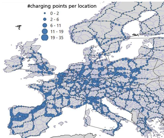
**Figure 2.** Proposed megawatt charging station locations for trucks in Europe. The map shows a potential public megawatt charging station network with stations located along the main European motorways at 50 km intervals. The size of the circles indicates the number of megawatt chargers that might be required at each location by 2030 or shortly after — depending on the future share of battery electric trucks. Figure taken from ref 21.
