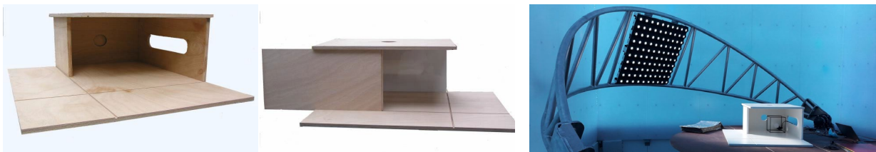
Figure 28. The principle of a "lumbox" and a "lumbox" under the sun-sky simulator.
