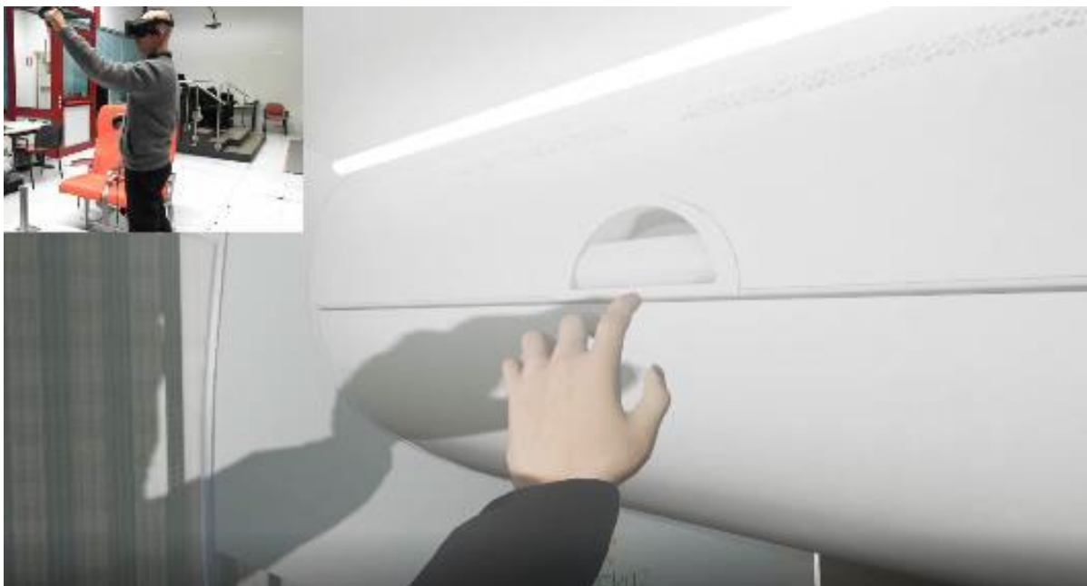
Figure 12. Stowage Bin opening test (real/virtual user coupled view).
