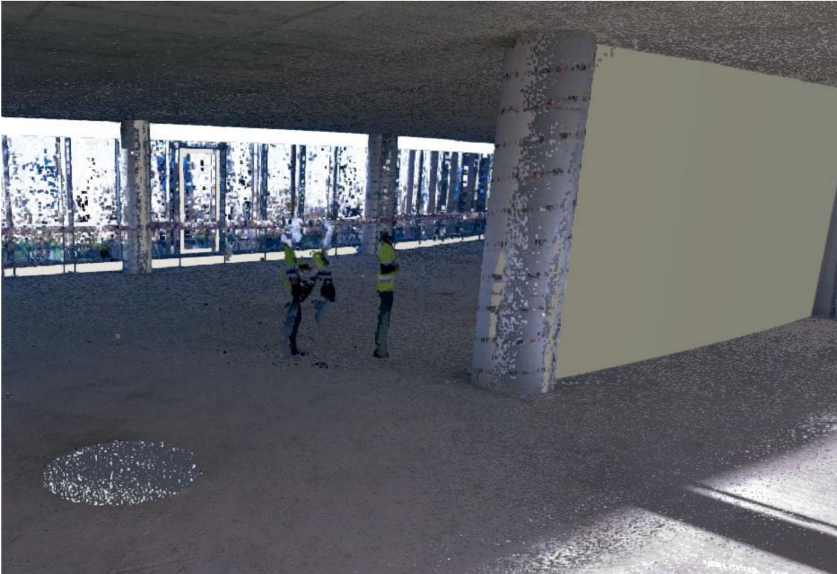
Figure 43. Example of captured data with wheeled robot on BIMprove pilot site in Madrid. Captured data can be shown together with the 3D model.
