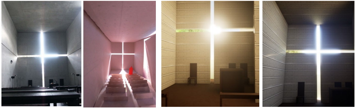
Figure 27. Tadao Andō's Church of the Light in real life, in physical model under the sky-sun simulator and two images of lighting simulation in virtual reality.
