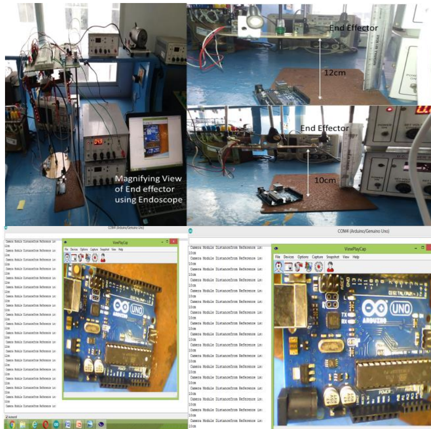
Figure 11. The Endoscopic magnified view with position feedback of ultrasonic sensor
