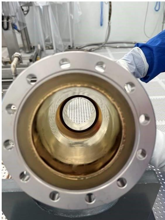
*Figure 5: visual inspection of a 1.3 GHz Nb cavity after ALD synthesis of a multilayer:  $\text{AlN/NbTiN}$ .*
