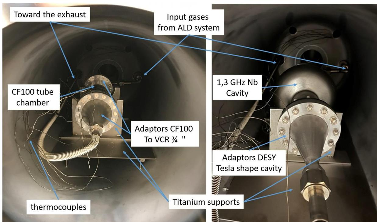
Figure 3: chamber (left) and cavity (right) installed inside the oven retort with adaptors.
