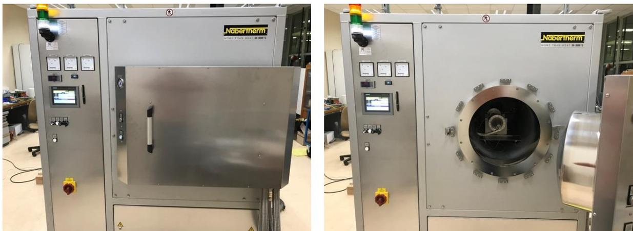
*Figure 2: front views of the vacuum Oven with retort door closed or open.*
