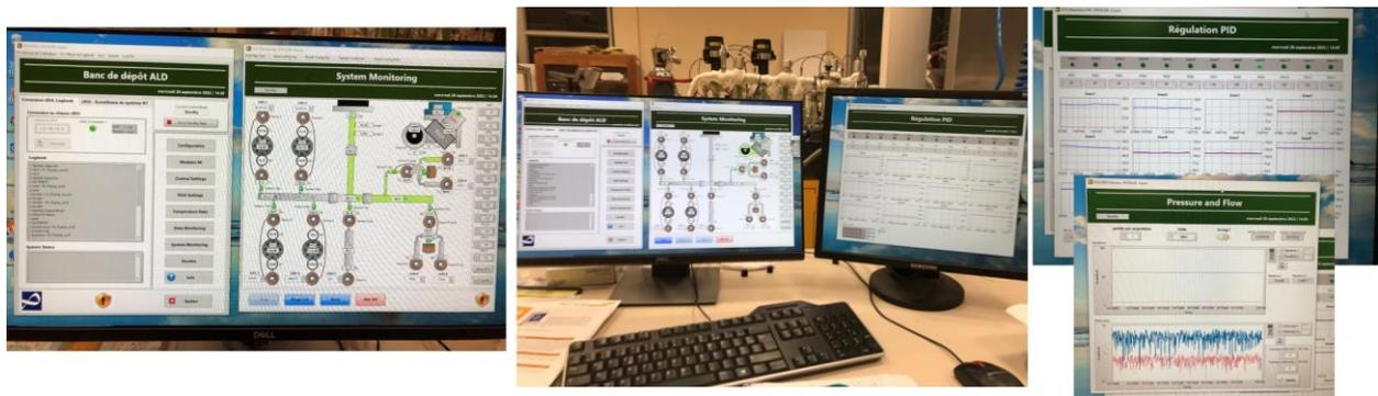
*Figure 4: Labview control program. Left: schematic of the ALD precursor delivery system where is displayed the zones temperature and pneumatic valves status. Right: Pressure and flow control windows being monitored during an ALD process.*
