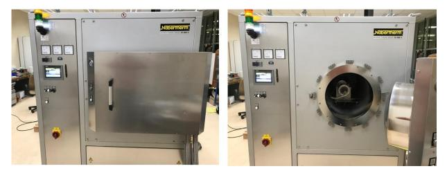
Figure 2: front views of the vacuum Oven with retort door closed or open.
