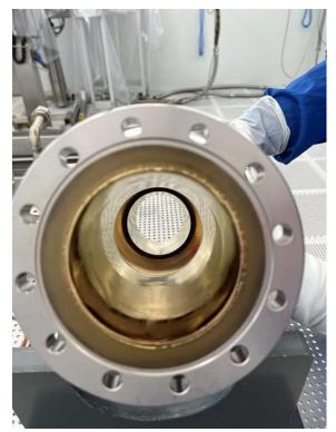
Figure 5: visual inspection of a 1.3 GHz Nb cavity after ALD synthesis of a multilayer: AlN/NbTiN.
