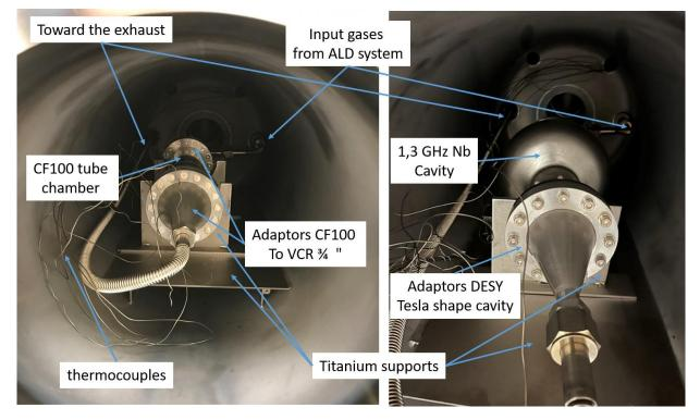
Figure 3: chamber (left) and cavity (right) installed inside the oven retort with adaptors.
