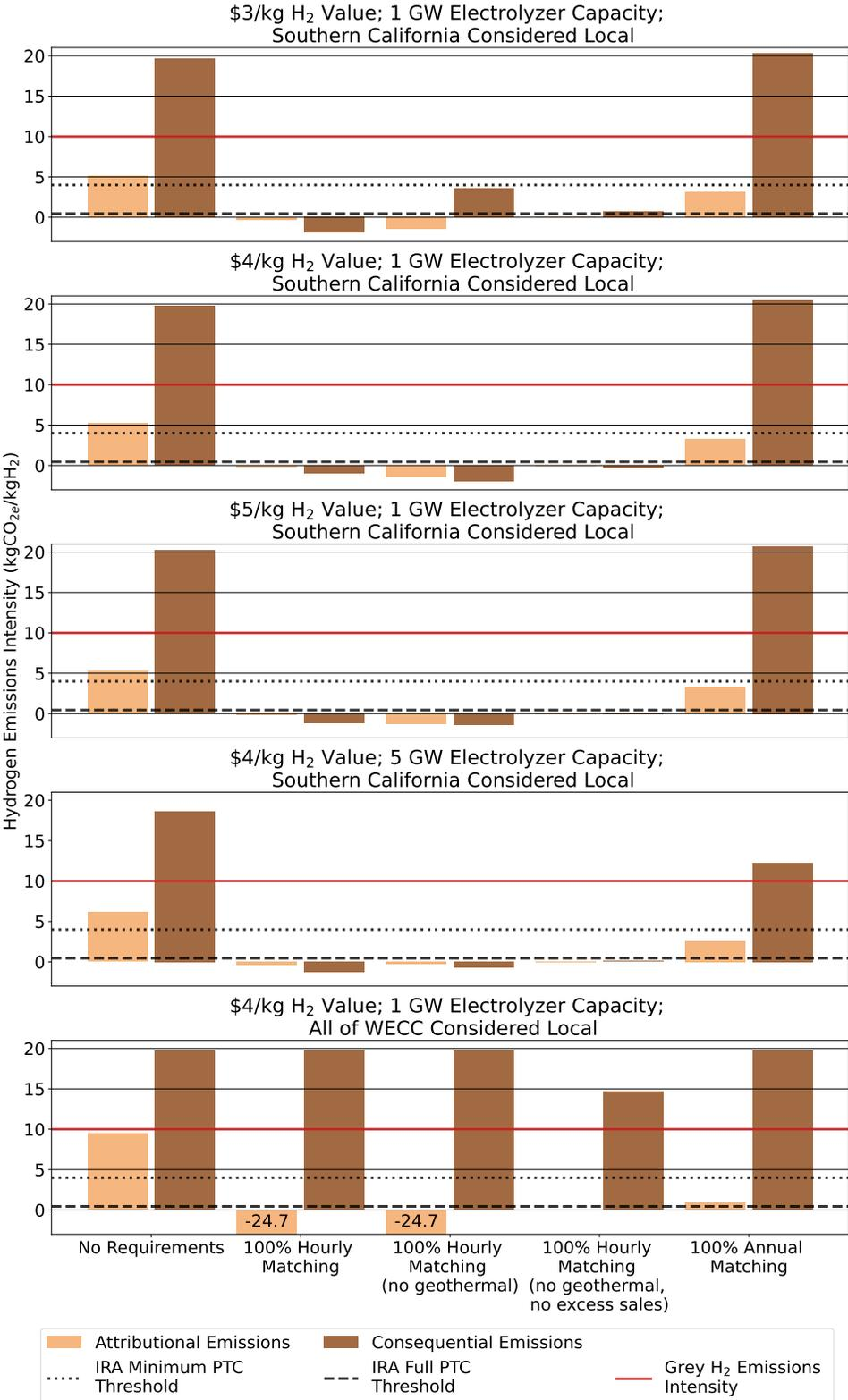
**Figure 2.** Attributional (left) and consequential (right) emissions rates from grid-produced hydrogen under a range of policy options and sensitivity scenarios.
