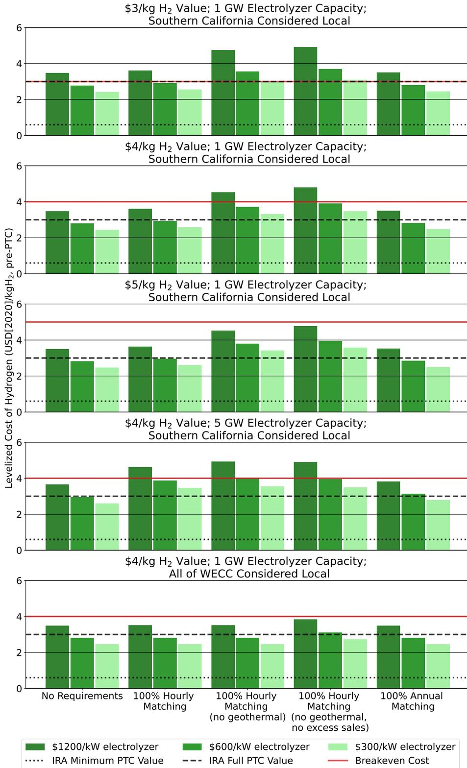
**Figure 5.** Levelized cost of hydrogen (LCOH) for production in southern California under the same scenarios shown in Figures 2 and 3, compared with potential revenues from sales. LCOH values are provided for a range of potential electrolyzer capital costs.
