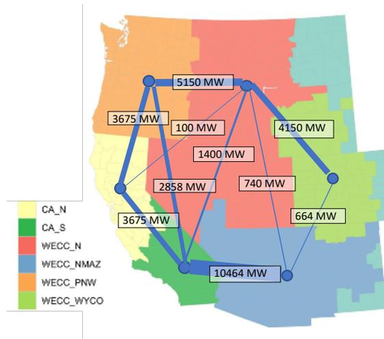
**Figure 1.** Illustration of the modeled U.S. Western Interconnection electricity system and its component zones, which represent single regions or aggregations of regions from the EPA’s Integrated Planning Model [25]. California is divided into two model zones. Existing interregional transmission capacities at the beginning of the planning period are shown.
