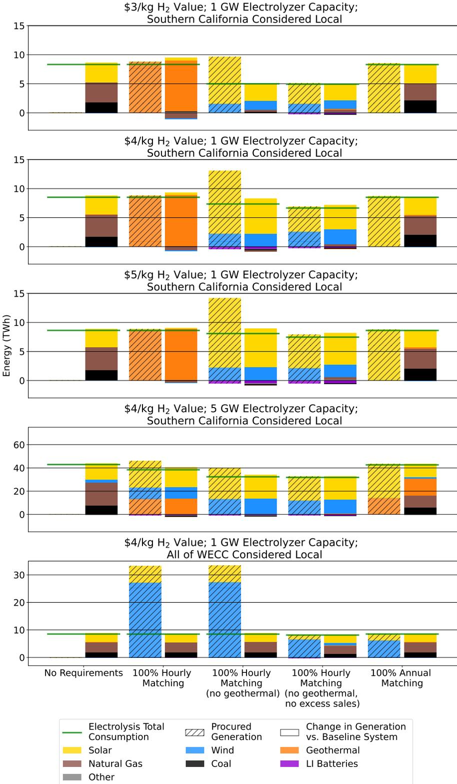
**Figure 3.** Total electricity consumption by hydrogen producers (green lines), compared with procured clean generation (left) and the actual observed changes in generation used to supply the additional hydrogen demand (right), under the same scenarios shown in Figure 2.
