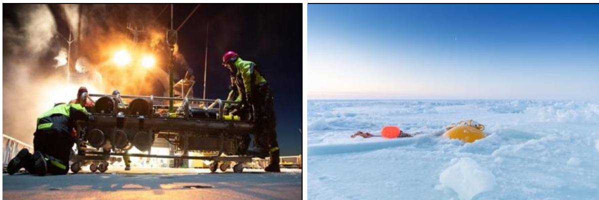
Figure 3: To the left: The temperature was -40^{\circ}\text{C} during the recovery of SIO-1 mooring and the photo to the left shows the acoustic source safely back on deck. To the right we see the top of the last mooring (SIO-3) which was trapped under the ice. It took 2 days with intense effort to recover this last mooring. In the end Coast Guard officer Andreas Soløy dived to located and rescue the mooring. All instruments were saved. (Photos: D. Fatnes, KV Svalbard)
