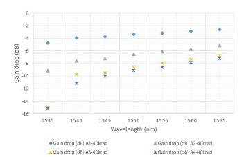
Fig. 3. Stage-1 post-irradiation optical gain drop as a function of wavelength for -45 dBm input power.
