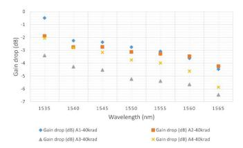
Fig. 4. Stage-1+2 post-irradiation optical gain drop as a function of wavelength for -45 dBm input power.
