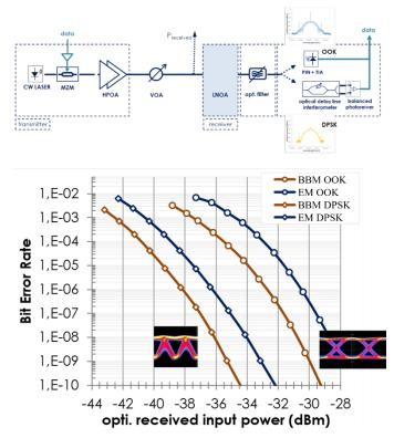
Fig. 7. (top) Schematic of optical transmission testbed, (bottom) BER measurements using the BBM and EM units as the LNOA for OOK and DPSK modulation format
