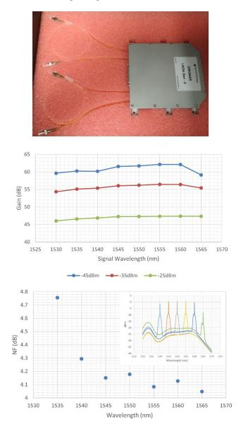
The amplifier measurements were obtained for a pump laser driving current equal to the maximum de-rated current, which is defined as 80% of the laser kink-free current.
