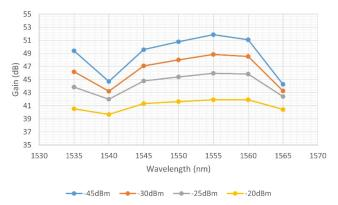
Fig. 2. Stage-1+2 pre-irradiation optical gain as a function of wavelength and input power for FOSA deploying sample A1.
