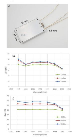
Fig. 5. (top) BBM optical pre-amplifier unit, (middle) optical gain as a function of wavelength and input power at the amplifier output and (bottom) NF as a function of input signal wavelength. The inset shows the optical spectrum trace at the amplifier output for 1540 - 1565 nm wavelength range.
