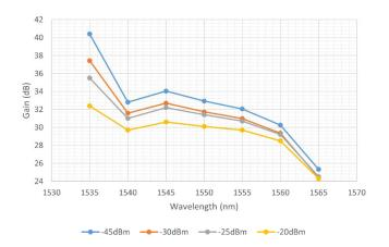
Fig. 1. Stage-1 pre-irradiation optical gain as a function of wavelength and input power for FOSA deploying sample A1.
