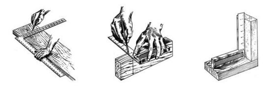
3. Marking gage was used for marking lines parallel to a surface of wood stock.
