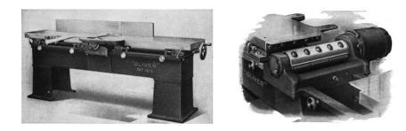
5. *Planer or surfacer* used mainly for finishing surfaces of flat stock and reducing stock to thickness. The more common type planes one surface at a time and is referred to as a single surfacer.
