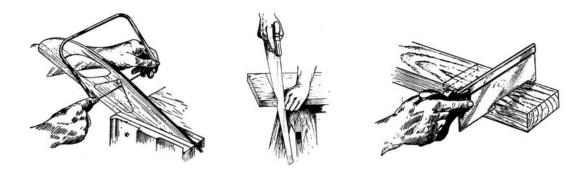
15. *Scraper* very useful in smoothing surfaces having the grain running in various directions, where a plane could not be used.
