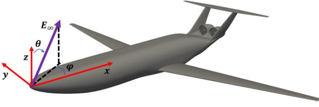
Figure 1. Coordinate system for the problem. Model aircraft is the MIT D8, to be discussed in Section 5.
