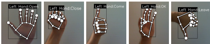
Fig. 4: Signs considered during Handover . From left to right: open , close , come , ok , and leave .
