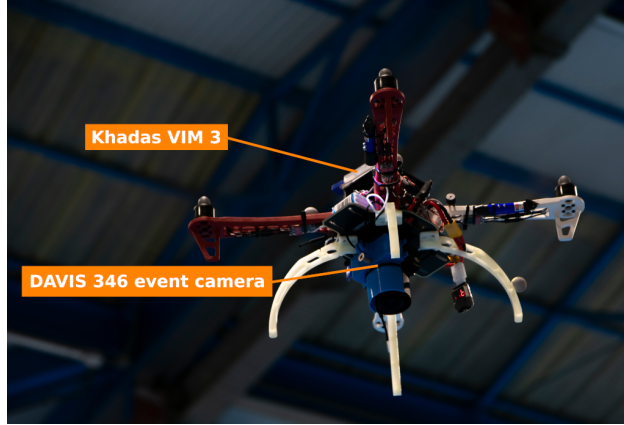
Figure 1: Aerial robot based on DJI Flamewheel F450 equipped with a DAVIS 346 event camera and a low-cost Khadas VIM3 used for on-board computation.
