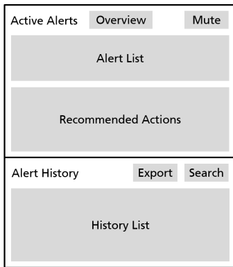
Fig. 2. Schematic layout of CIM’s HMI with two main sections for active cyberalerts including decision support (top), and cyberalert history (bottom).
